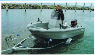
was configured as a centre console, with a large chilly bin camouflaged as a bench seat providing seating for two amidships. A tiller-steered configuration is also possible for this hull. As indicated by the model designation, the hull is 4.2m in length, with a maximum beam of 1.93m.
