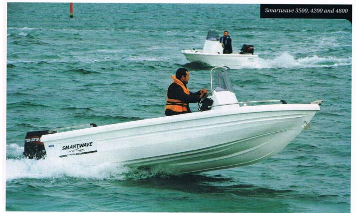
ABOVE The more conventional vee hull of the 4800 tracks flat, while the extra weight helps punch through chop. RIGHT Moulded drinkholders are a handy addition; the 50hp Tohatsu had the lightweight polyethylene hull boogeying at more than 20kts.
