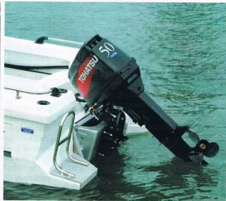
This gives enough stability for the boat to be rated for five people, despite its modest size. Yet at speed, the hull lifts enough to smooth out the ride without losing stability. The hull acts to contain the spray generated by the bow, turning it down to create a relatively dry ride.
